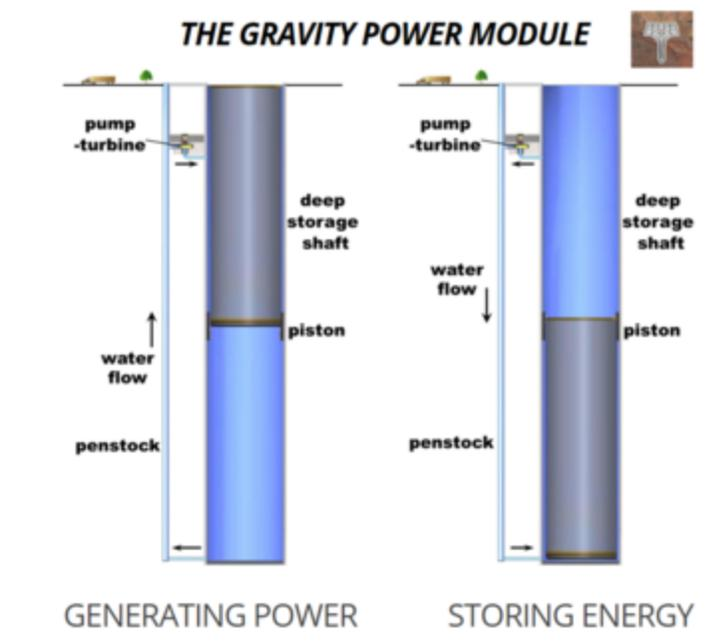
As an example of the potential performance of gravity energy storage, 1,200MW delivered across 4.6Hrs can be secured from a hole 700 meters deep and 30 meters wide.
